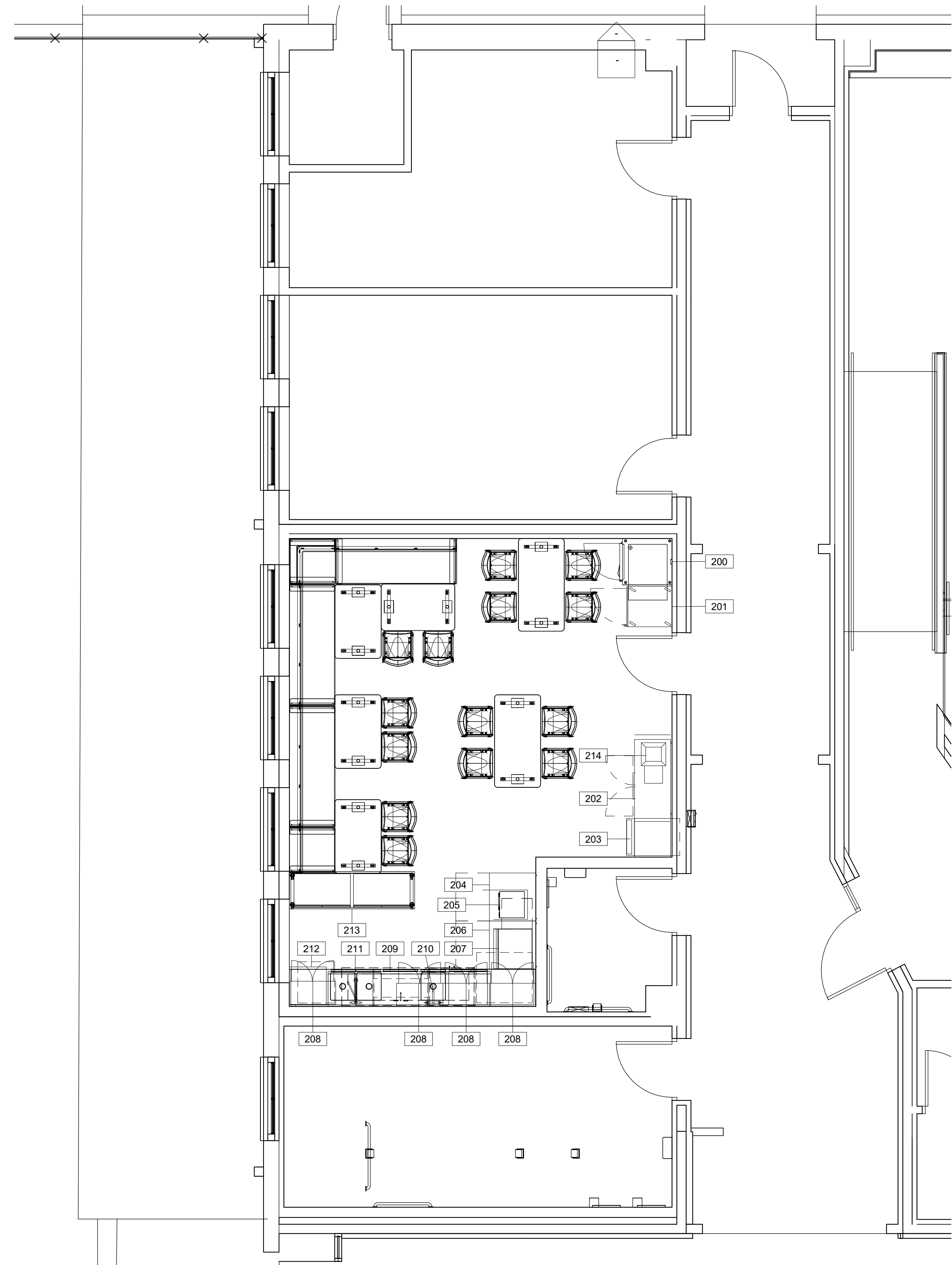
① LEVEL 1 - WARMING KITCHEN EQUIPMENT PLAN 1/4" = 1'-0"
